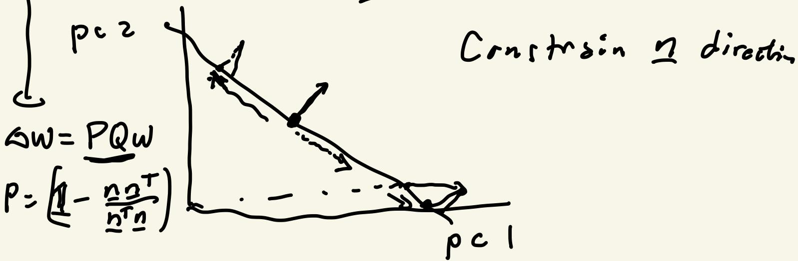
$$\Delta \underline{w} = Q \underline{w} + \text{multiply to set } \sum_i w_i = c$$
